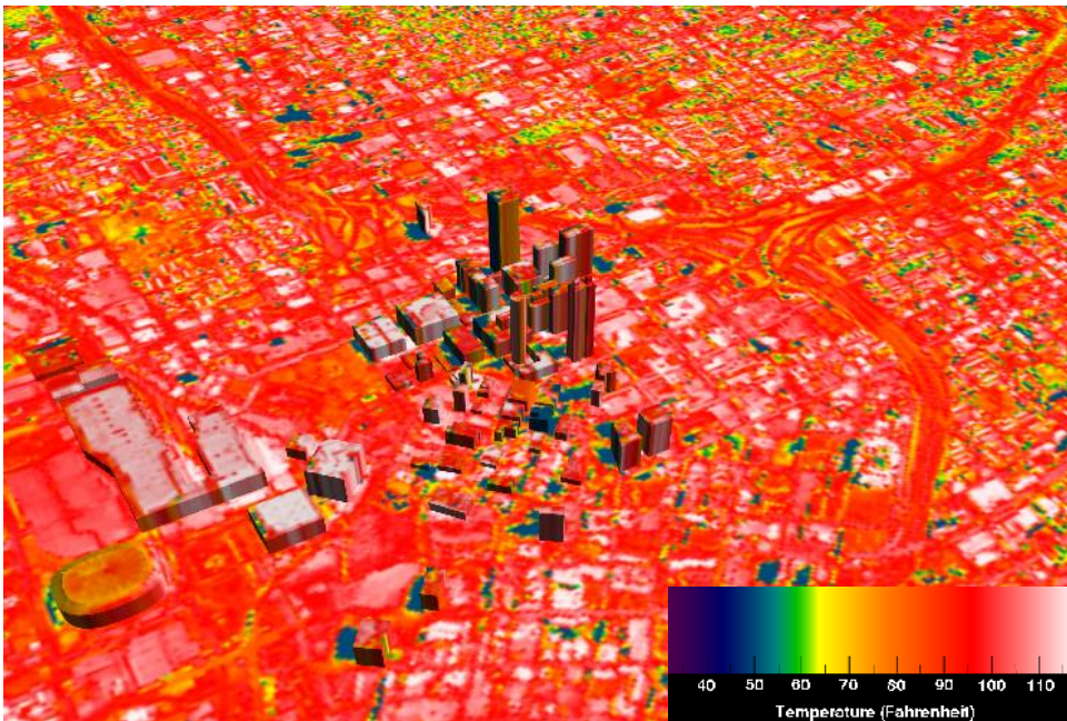
Picture 1: Atlanta, GA, Daytime Thermal View of the Heat Island
